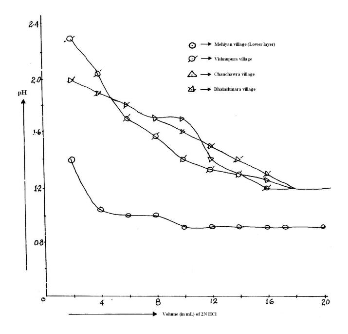
$Figure-2 \\ Comparative\ Titration\ Curve\ of\ pH\ value\ against\ sample\ solution\ of\ lower\ layer\ solid\ solutions\ with\ 2(N)\ HCl$
