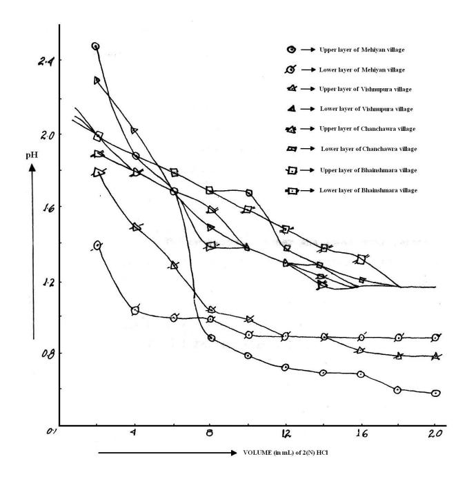
Figure-3 Comparative Titration Curve of pH value against sample of upper and lower layer solid solutions with 2(N) HCl
